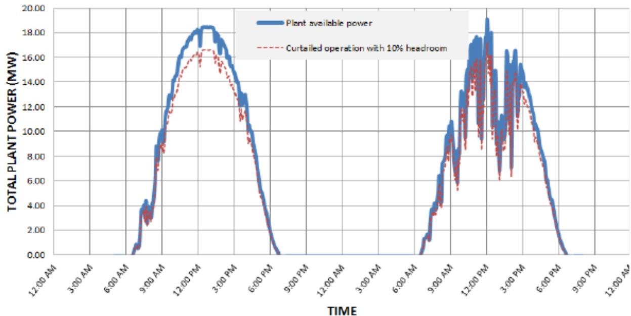
**Figure 98. Total power of the Illumina PV power plant with reserve over two days with different weather (August 3<sup>rd</sup>, 4<sup>th</sup> 2014). The red curve indicates a potential 10% curtailment (Gevorgian & O’Neill, 2016).**
