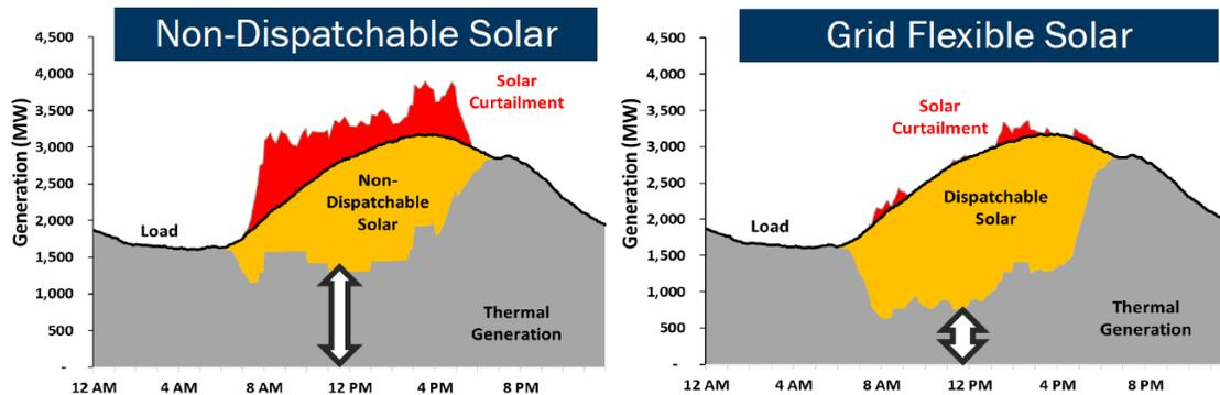
Figure 100. Illustration of how grid flexible solar reduced curtailment and thermal generation around noon (Loutan et al., 2017).
