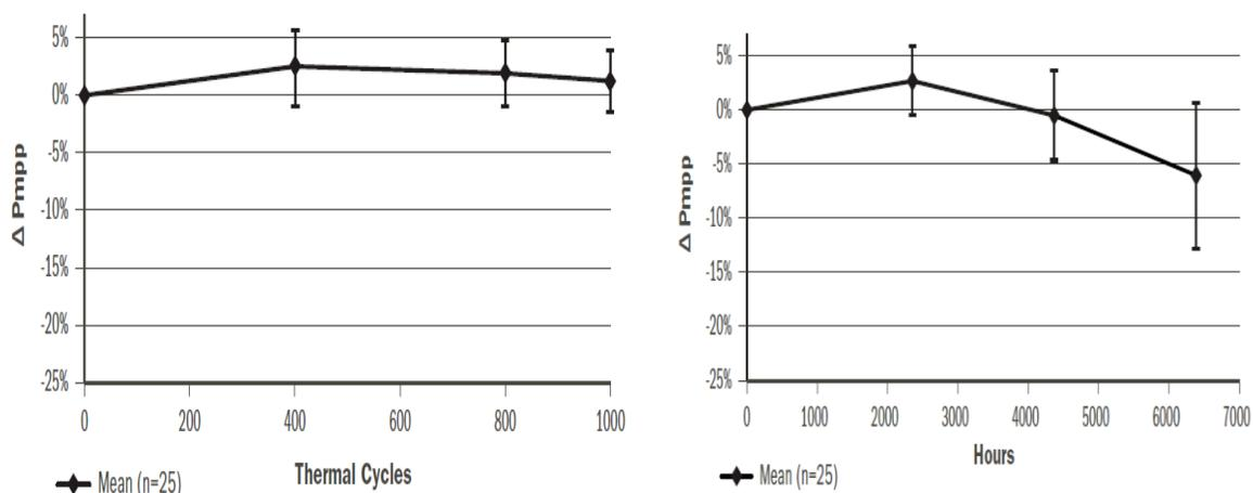
**Figure 41. Left - result of extended thermal cycling. Right - Result of extended damp heat testing. Testing durations are five times for thermal cycling, and more than six times that of standard procedures for damp heat testing. No power reduction was observed for thermal cycling, during damp heat testing, power reduced by only about 7%, despite the harsh testing conditions (Strevel et al., 2013).**
