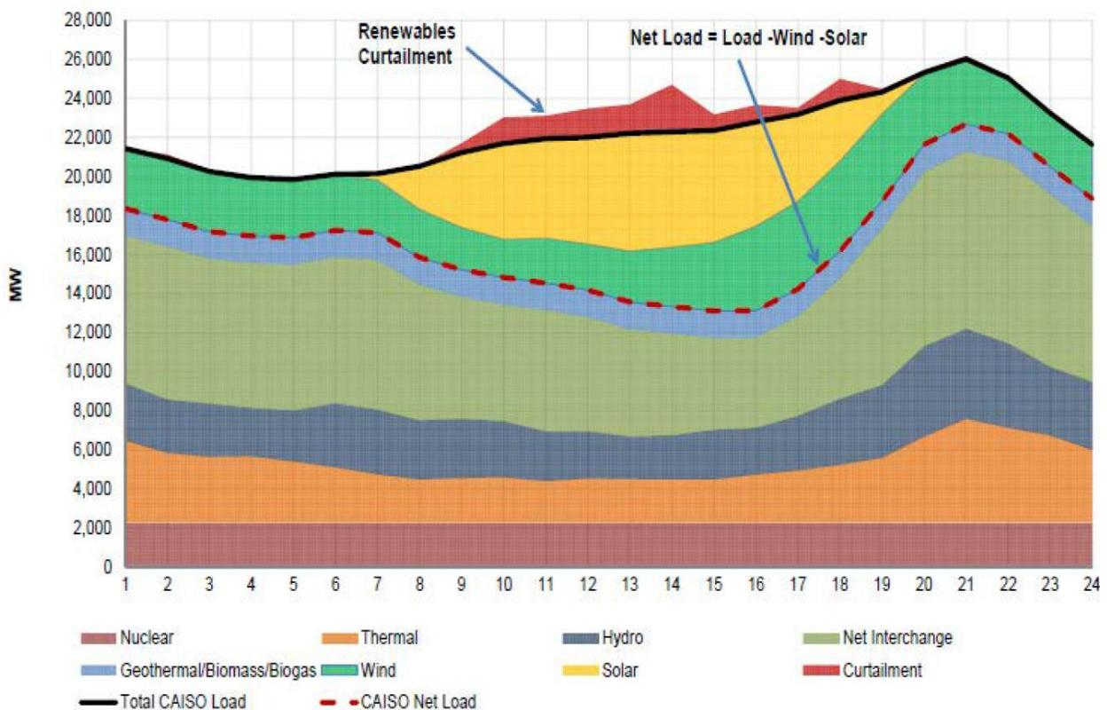
**Figure 99. Load profile for California (CAISO) on April 24<sup>th</sup> 2016. Also shown are the different contributors (Loutan et al., 2017).**
