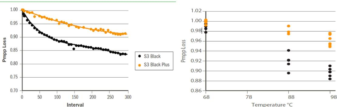
Figure 43. Left - Power loss after extended light soaking exposure. The ZnTe-based device (Series 3 Black Plus) showed less than 10% reduction after 300 days of testing. Right - Comparative power loss vs. accelerated temperature and light soaking stresses. The improved long-term stability of the ZnTe-based device (Series 3 Black Plus) is an indication of inhibited Cu migration due to the presence of ZnTe (Strevel et al., 2013). Note that ZnTe is also utilized in Series 4|6 modules.
