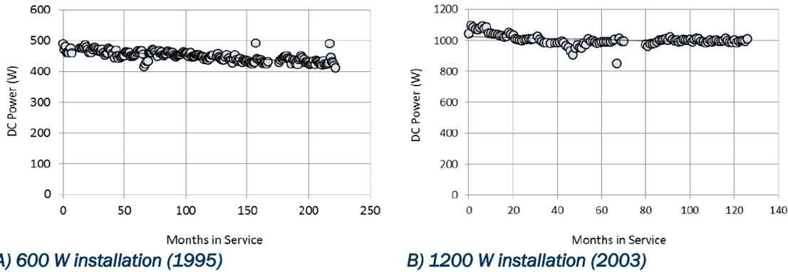
**Figure 28. A) DC Power output over 19 years for a 600 W CdTe research module installation from 1995. B) DC Power output over 10 years for a 1200 W CdTe research module installation from 2003. The latter module is technologically close to First Solar’s modules (Ngan et al., 2014).**
