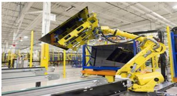
*Figure 60. Automated manufacturing process for First Solar Series 6 manufacturing.*
