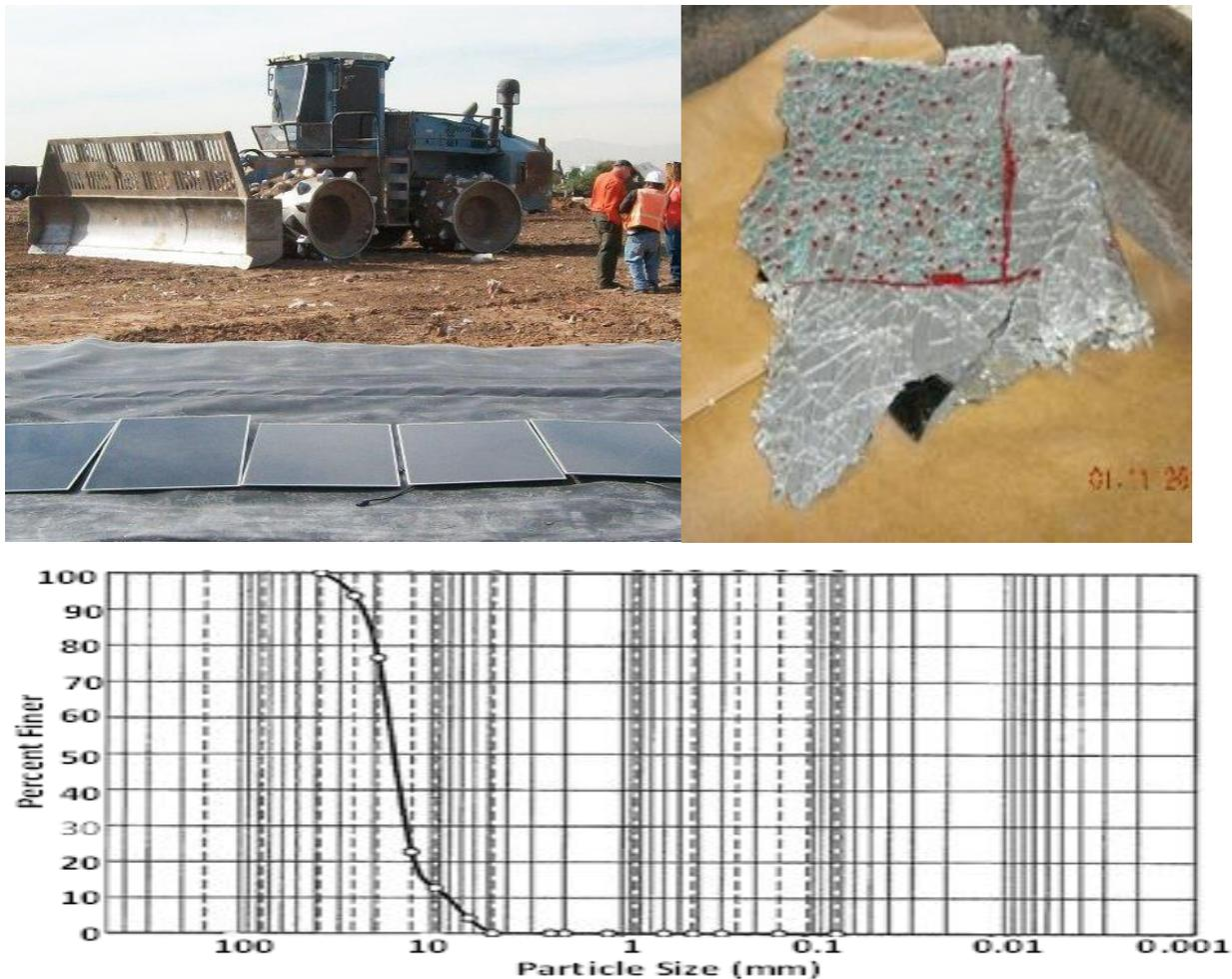
*Figure 71. Landfill compactor used to crush PV modules in a municipal landfill in Arizona (top left) and compactor foot punch out (top right) and PV module fragment size distribution (bottom) (Sinha et al., 2014).*
