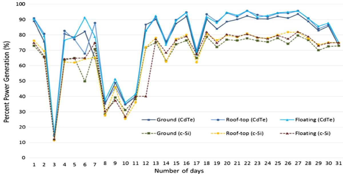
**Figure 36. One-month comparison of Cadmium Telluride and polycrystalline silicon PV modules on different installation. Considered are ground-mounted, rooftop and floating PV systems (Munshi et al., 2018).**
