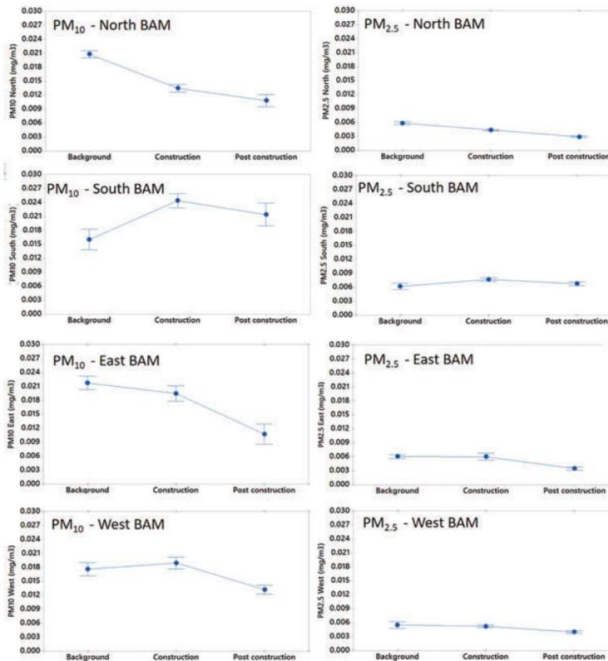
Figure 91. Particle concentration (PM<sub>10</sub>-PM<sub>2.5</sub>) before, during and after construction including confidence intervals of 95%. Taken from beta attenuation monitor stations around the PV plant (Ravikumar & Sinha, 2017).
