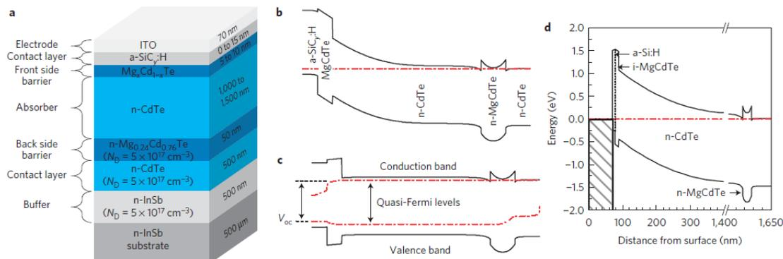
**Figure 48. A) Device structure of a CdTe solar cell that incorporates Magnesium for band gap grading. B) and C) Show the band structure qualitatively of this device in the dark and under illumination. D) Shows the calculated absolute energy (Zhao, 2016).**
