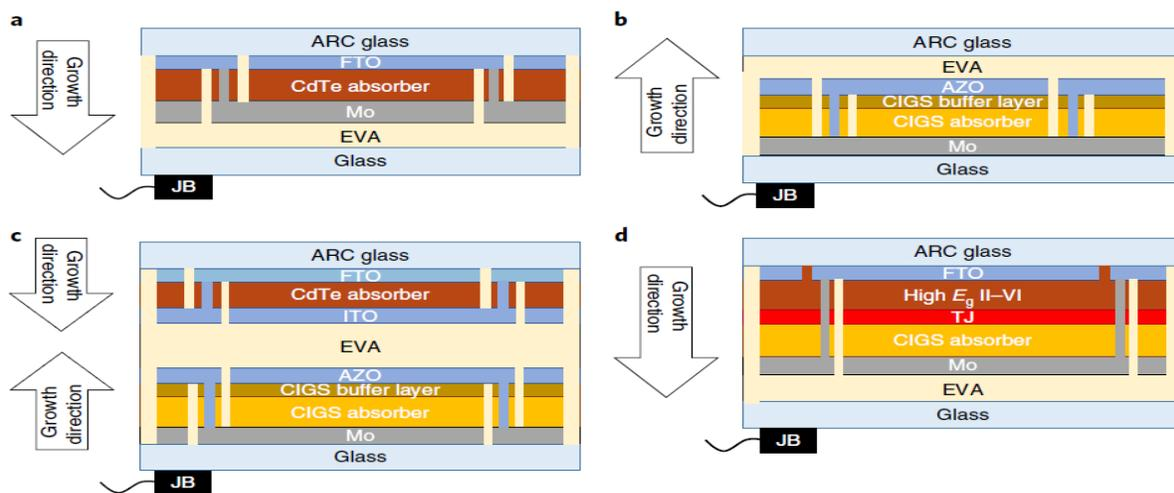
**Figure 51. Cell structures explored in a comparison of single junction and tandem solar cells in the U.S. market (Sofia et al., 2018).**
