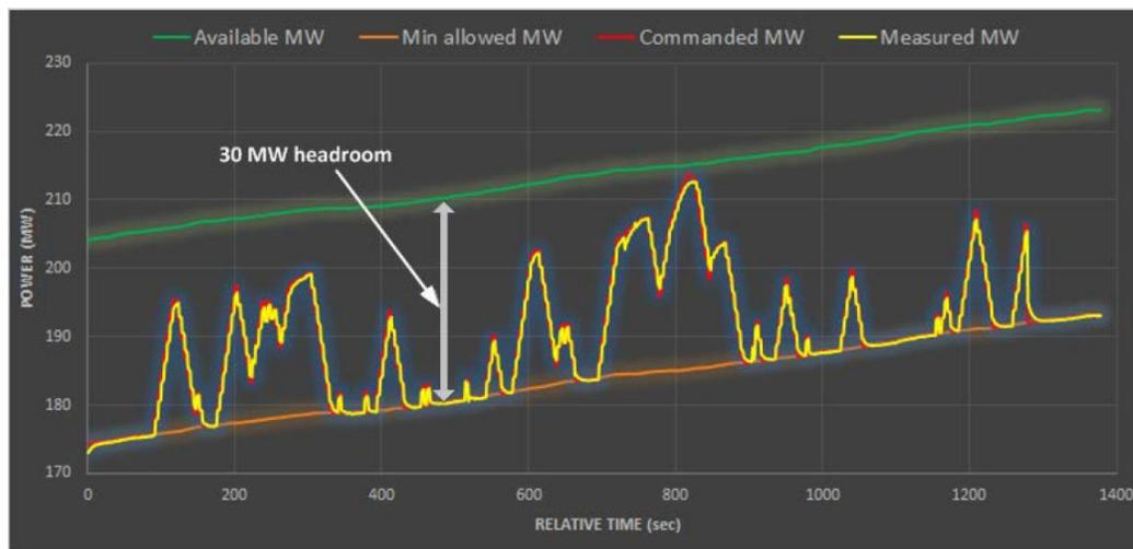
**Figure 102. Experimental validation of automated generation control (AGC). The figure shows the power output profile of a First Solar 300MW power plant with CAISOs footprint on August 24<sup>th</sup> 2016 between 9:47 and 10:10 (Loutan et al., 2017).**
