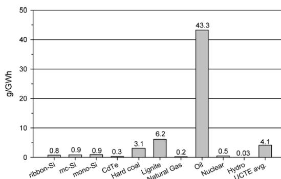
FIGURE 3. Life-cycle atmospheric Cd emissions for PV systems from electricity and fuel consumption, normalized for a Southern Europe average insolation of 1700 kWh/m<sup>2</sup>/yr, performance ratio of 0.8, and lifetime of 30 yrs. Ground-mounted BOS (18) is assumed for all PV systems; comparisons with other electricity generation options.
