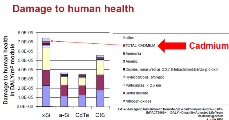
Cadmium emissions to air by CdTe PV module production contribute
