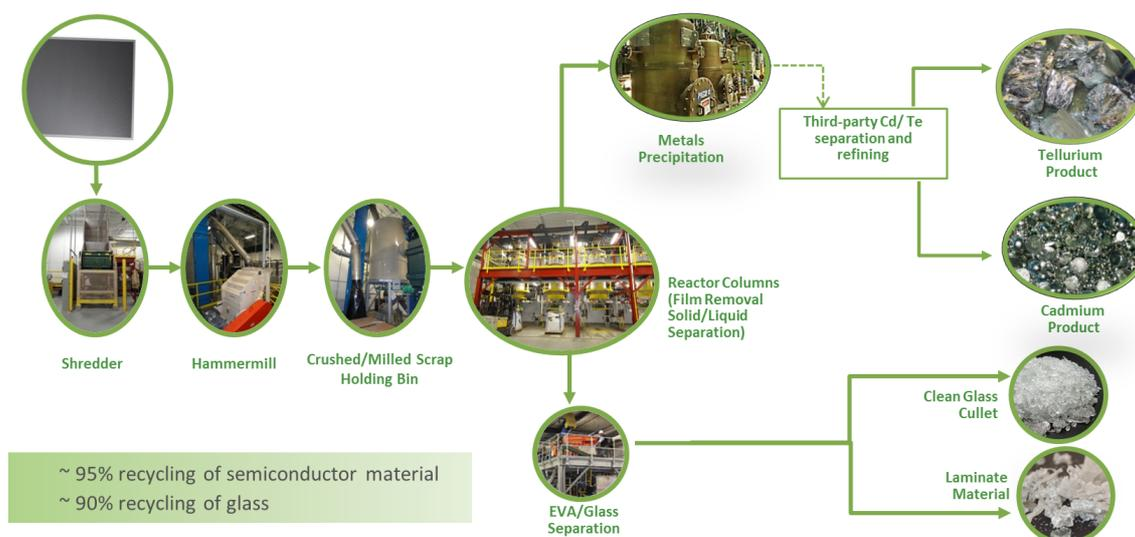
**Figure 4** First Solar's module recycling technology version 2
