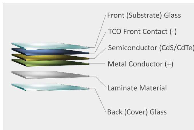
**Figure 2** Schematic representation of First Solar module architecture<sup>12</sup>
