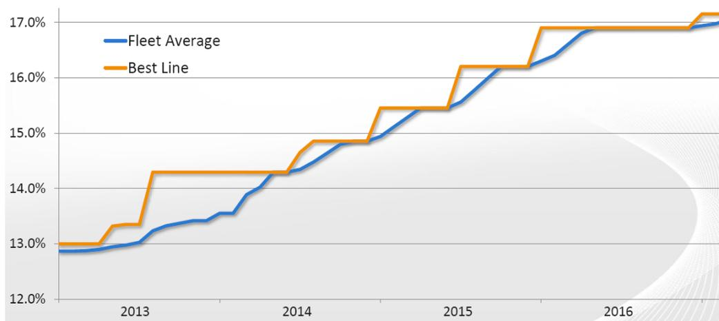
**Figure 10** First Solar CdTe module efficiencies roadmap
