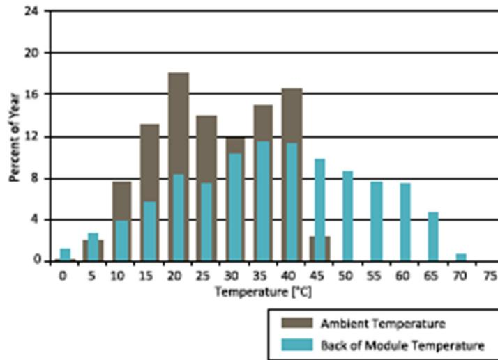
Figure 29: Distribution of ambient and back-of-module surface temperatures measured in a First Solar PV array in the USA desert Southwest area [58].
