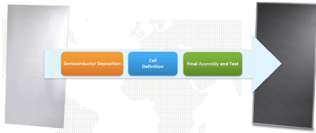
Figure 16: Conceptual and simplified flow of First Solar CdTe manufacturing process, from glass to finished PV module, in which all process steps are carried out at the same manufacturing plant.
