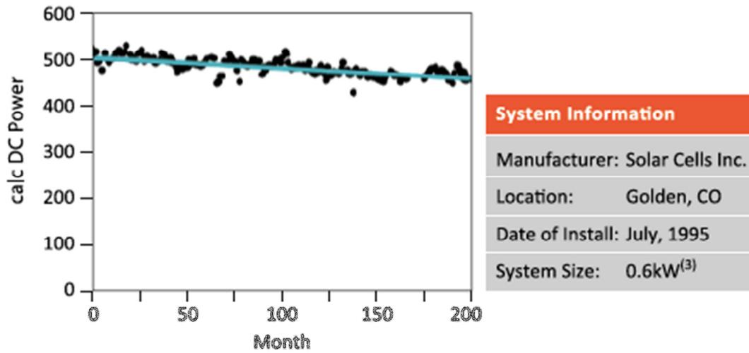
Figure 36: Long-term performance assessment of First Solar (formerly Solar Cells Inc.) CdTe PV modules carried out by the National Renewable Energy Laboratory – NREL, from 1995 to 2012. Annual output power degradation rate is 0.53%/year [58].
