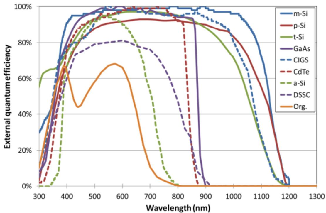
Figure 7: External quantum efficiency curves for a number of solar cell materials. The more shifted to the left (lower wavelengths) a curve is, the better the corresponding material will respond to a blue-shifted spectral content of light [37].
