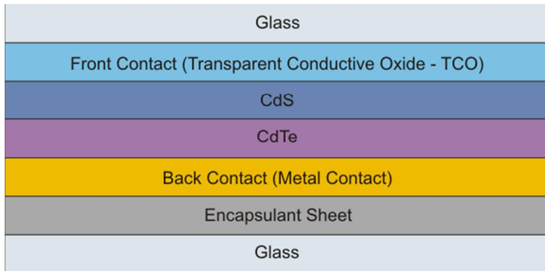
Figure 5: Schematic structure (layer thicknesses not to scale) of First Solar's thin-film CdTe PV devices, showing the active CdTe and CdS semiconductors, and metal and oxide (back and frontal) contacts sandwiched between two sheets of glass.
