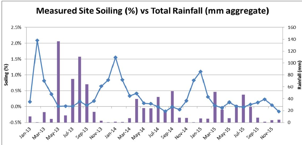
**Figure 2: Measured loss due to soiling at GRSF (GRSF, 2016)**
