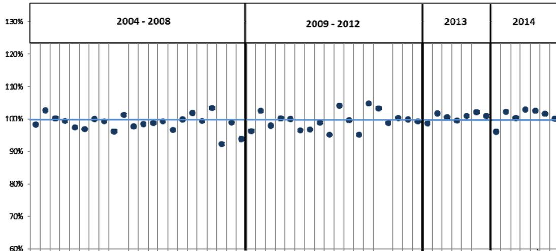
**Figure 1: Average Predicted Energy Ratios of First Solar plant by commissioning date (Strevel, 2015)**
