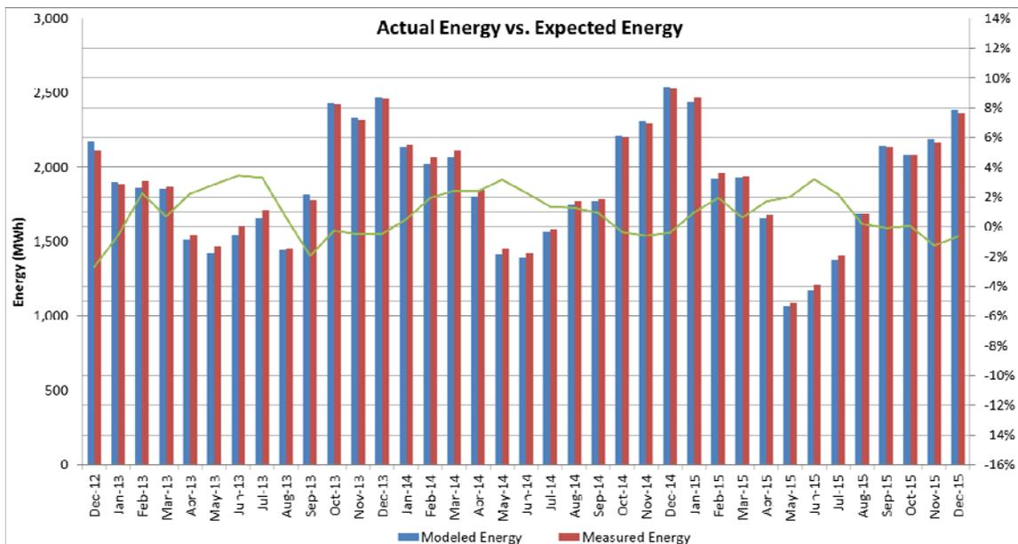
**Figure 6: Actual vs Expected Performance for GRSF, adjusted for soiling, spectrum, weather, and outage lost energy (GRSF, 2016)**
