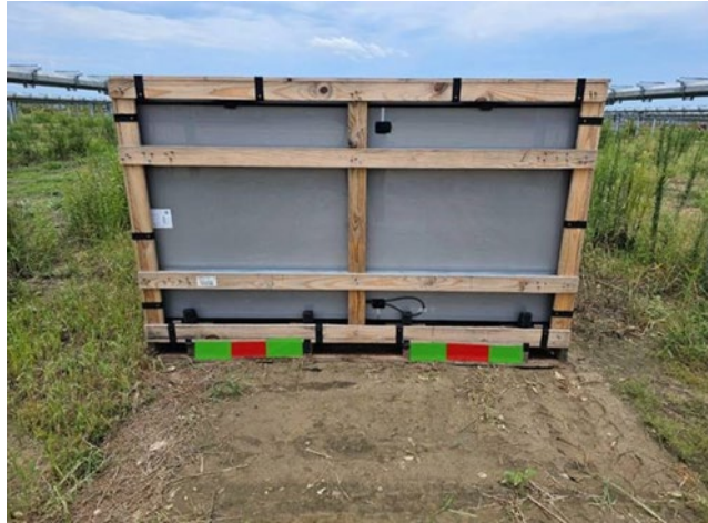
Figure 1: Correct Engagement Points for Lifting Pack from Long Side
