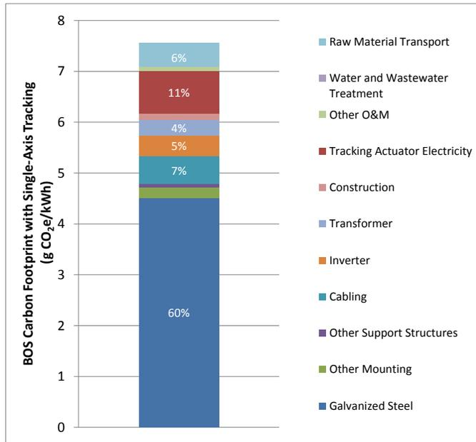
Fig. 4. BOS carbon footprint by component of CdTe PV single-axis horizontal tracking utility-scale systems. Based on Q4 2012 module conversion efficiency of 12.9%, 30 year lifetime, specific yield of 2162 kWh/kWp/yr, 0.70%/yr module degradation rate, and California grid (CAMX eGrid subregion).
