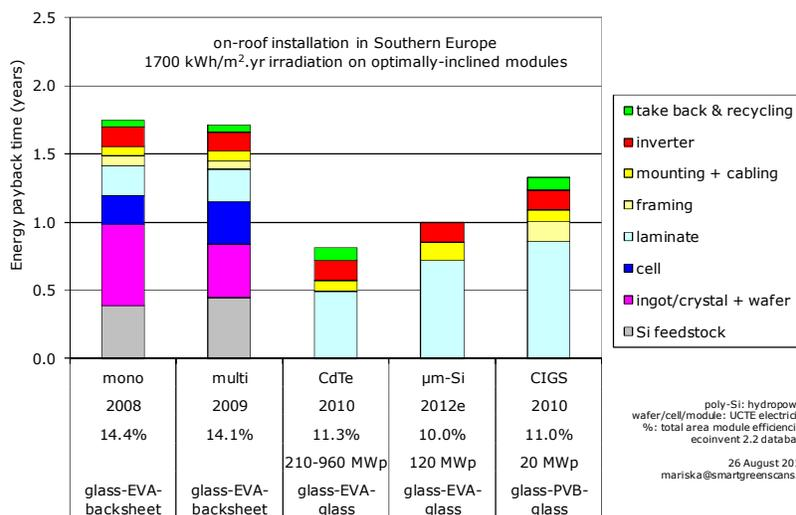
**Figure 4.** Energy payback time of commercial PV systems installed on roof-top at irradiation of 1700 kWh/m<sup>2</sup>/year on optimally-inclined modules. The data for micromorphous silicon PV modules are estimates (de Wild-Scholten, 2011).
