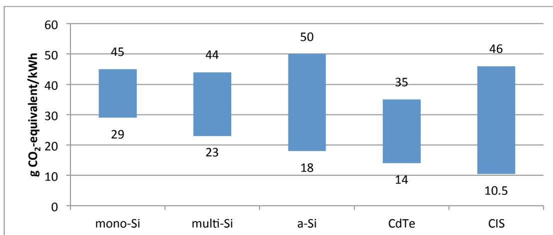
**Figure 13** GHG emissions for different PV technologies. Irradiation standardized at 1700 [kWh/m<sup>2</sup>/yr]. Adapted from Peng et al., 2013.
