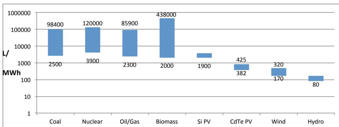
**Figure 18** Life cycle water withdrawal for different energy generation options (Sources: Fthenakis and Kim, 2010; Sinha et al., 2013)
