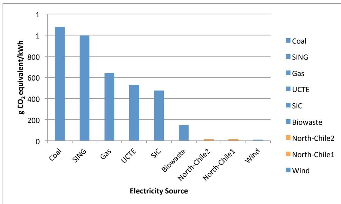
**Figure 15** GHG emissions [g CO<sub>2</sub>-eq./kWh] for different electricity sources.
