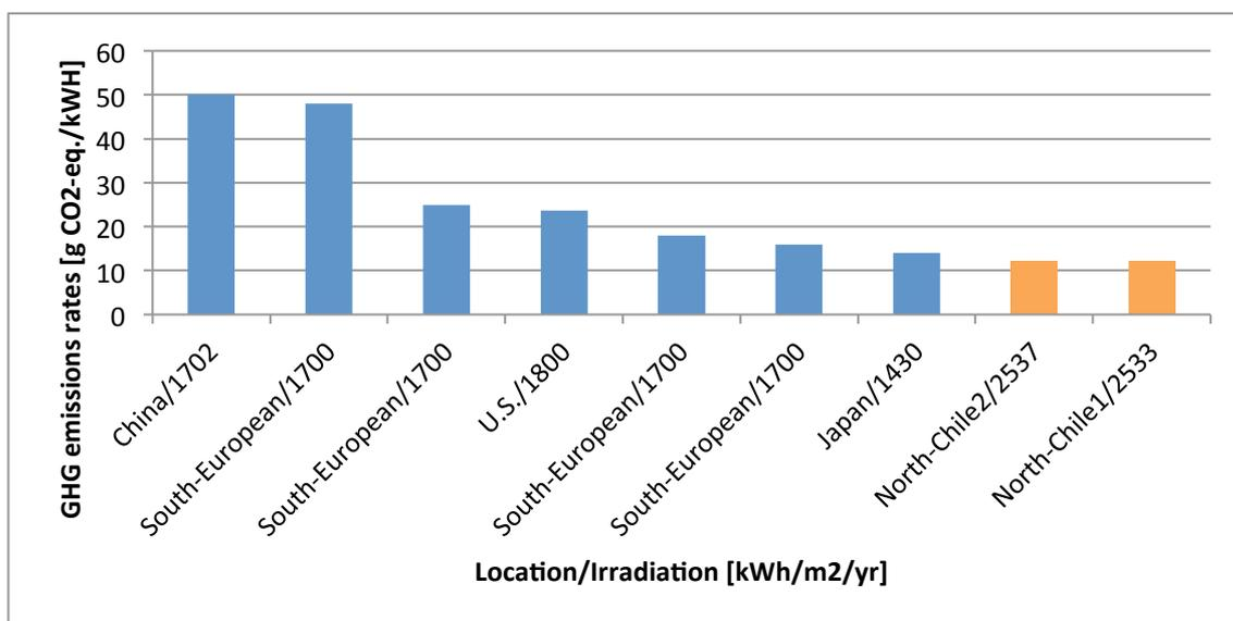
Figure 14 GHG emissions [g CO<sub>2</sub>-eq./kWh] for different PV technologies and irradiances<sup>25</sup>.
