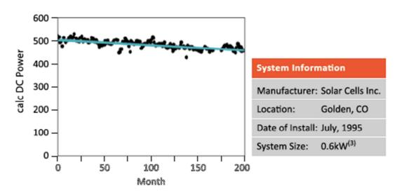
Figure 36: Long-term performance assessment of First Solar (formerly Solar Cells Inc.) CdTe PV modules carried out by the National Renewable Energy Laboratory – NREL, from 1995 to 2012. Annual output power degradation rate is 0.53%/year [58].
