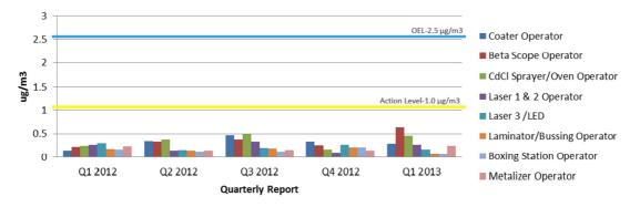
Figure 18: Personal exposure to Cd at First Solar manufacturing plants for the various stages of CdTe PV module production.
