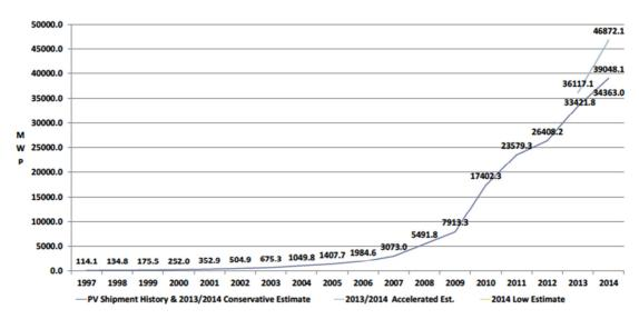
Figure 2: Global PV shipments from 1997 to 2014 [30]. With the PV incentive programs that were started with the establishment of the German feed-in tariff in the early 2000's, the global PV market reached the necessary scale for an effective cost-reduction that is still in course.
