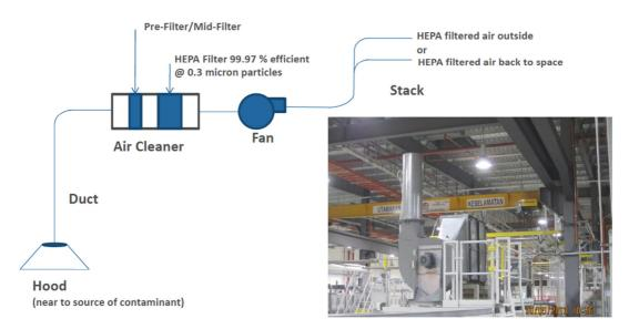
Figure 24: First Solar's CdTe PV module manufacturing plant Local Exhaust Ventilation (LEV) system. The photo shows the High Efficiency Particulate Air (HEPA) filter's exhaust air being recirculated back to the manufacturing floor space.
