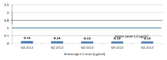
Figure 17: Cd levels routinely measured at the Malaysia KLM First Solar factory, which are well below the action limit of 1  $\mu$ g/m<sup>3</sup>.
