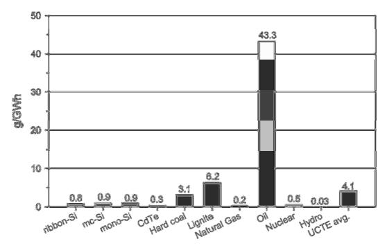
Figure 25: Lifecycle atmospheric Cd emissions for ground-mounted PV systems from electricity and fuel consumption for a Southern European average insolation of 1,700 kWh/m2/year, performance ratio of 0.8, and lifetime of 30 years [45].
