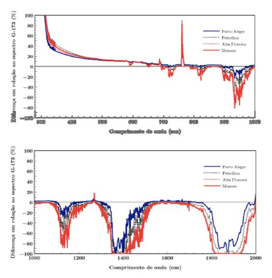
Figure 9: Relative difference between the spectral content of sunlight at four Brazilian sites, and the Standard ASTM G-173 spectrum, showing that the four locations have a spectral distribution that has more blue and less red photons than the standard spectrum [38].
