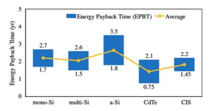
Figure 26: Energy Payback Times (in years) for commercially-available solar PV technologies [52].
