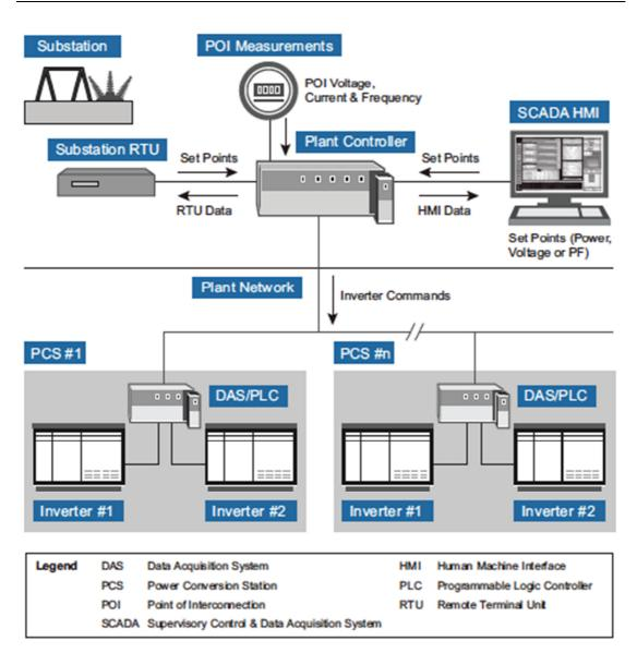
Figure 33: Example of a plant control system and interfaces to other components [67].
