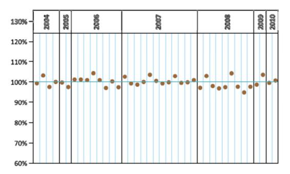
Figure 37: Average Predicted Energy Ratio – PER, by commissioning year, for 270MW of thin-film CdTe PV systems using First Solar modules: >270MW monitored installations base, including >130MW of hot-climate deployments [58].
