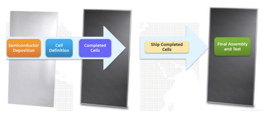
Figure 21: Conceptual and simplified flow of First Solar CdTe split line manufacturing process, from glass to finished PV module, in which some of the initial process steps are carried out at the base plant (PBG or KLM), and bundled single glass panes with completed cells are shipped elsewhere for final assembly and test at another manufacturing plant.
