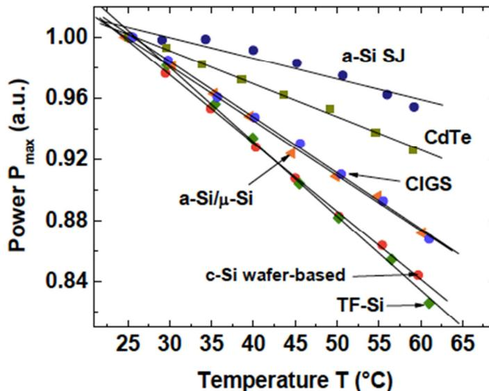
Figure 6: The negative effect of operating cell temperatures on the output power of first- and second-generation PV technologies [36].
