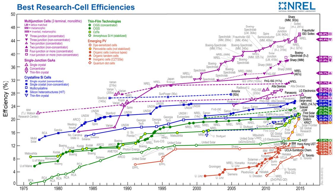
Figure 17: The National Renewable Energy Laboratory – NREL’s solar cell efficiency chart [29] showing the evolution of the best research-cell efficiencies since the 1970’s (updated June 2015).
