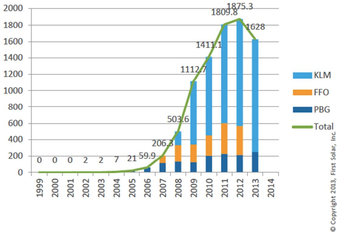
Figure 11: Annual PV module production (in MWpDC/year) for the three CdTe PV module manufacturing and recycling plants that First Solar runs in Perrysburg-OH (USA), Frankfurt-Oder (Germany) and Kulim (Malaysia).
