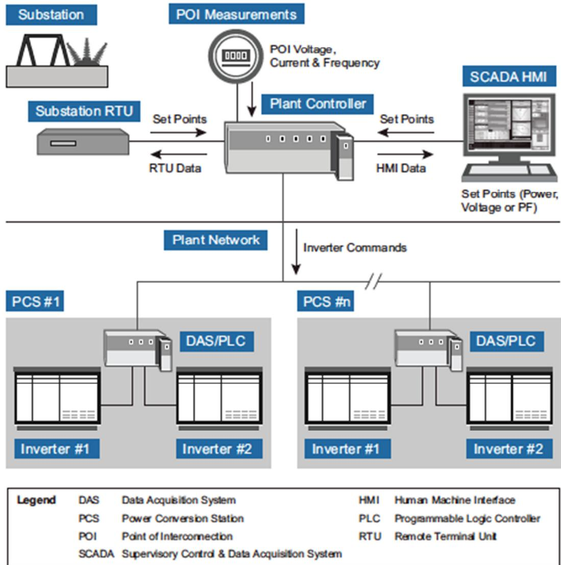
Figure 33: Example of a plant control system and interfaces to other components [67].
