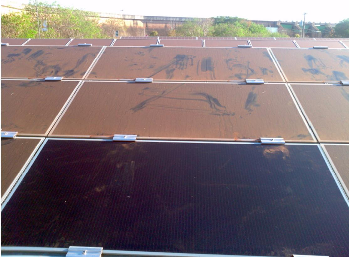
Figure 31: Example of heavy, uniform soiling conditions at a PV test site in the Brazilian Southeast.
