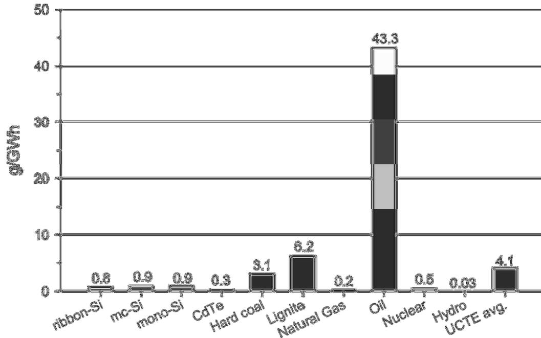
Figure 25: Lifecycle atmospheric Cd emissions for ground-mounted PV systems from electricity and fuel consumption for a Southern European average insolation of 1,700 kWh/m<sup>2</sup>/year, performance ratio of 0.8, and lifetime of 30 years [45].
