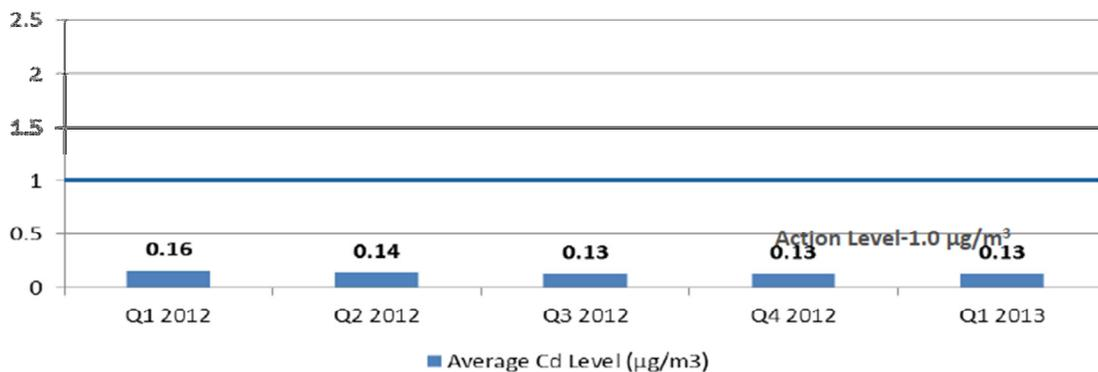
Figure 17: Cd levels routinely measured at the Malaysia KLM First Solar factory, which are well below the action limit of 1 µg/m<sup>3</sup>.
