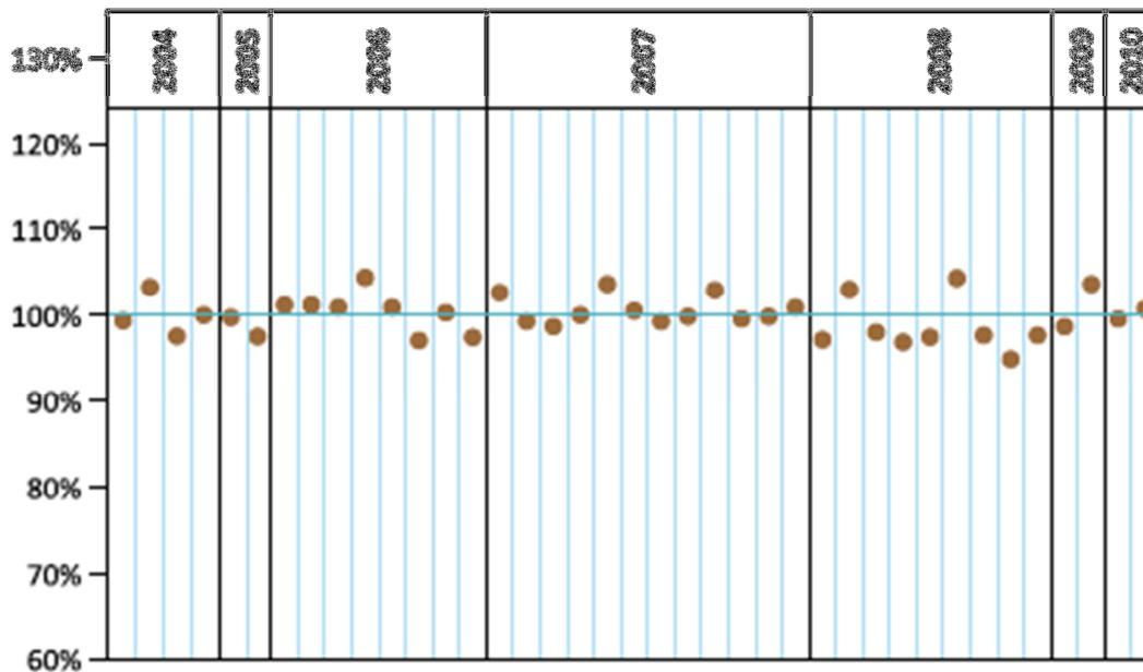
Figure 37: Average Predicted Energy Ratio – PER, by commissioning year, for 270MW of thin-film CdTe PV systems using First Solar modules: >270MW monitored installations base, including >130MW of hot-climate deployments [58].
