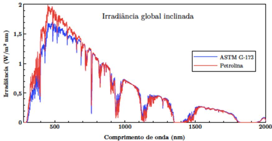
Figure 8: Spectral distribution of sunlight at the Brazilian site Petrolina-PE (latitude = 9o23'' South), in comparison with the Standard ASTM G-173 spectrum, showing the higher level of irradiance at lower (bluer) wavelengths at latitude tilted planes [38].
