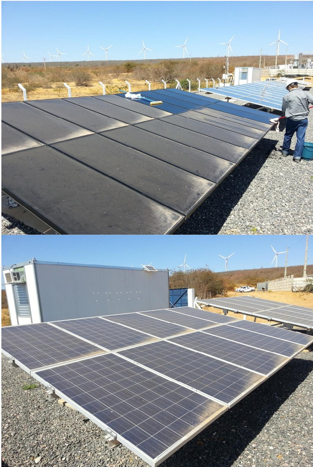
Figure 32: Examples of heavy, non-uniform soiling conditions at a PV test site in the Brazilian Southeast; non-uniformities in soiling patterns are mainly caused by strong wind conditions.
