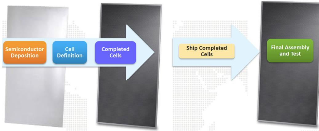
Figure 21: Conceptual and simplified flow of First Solar CdTe split line manufacturing process, from glass to finished PV module, in which some of the initial process steps are carried out at the base plant (PBG or KLM), and bundled single glass panes with completed cells are shipped elsewhere for final assembly and test at another manufacturing plant.
