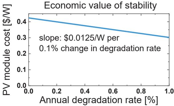
Fig. 1. Iso-LCOE plot (obtained with NREL SAM) displaying variations in PV module cost and annual degradation rate for achieving SunShot 2020 utility-scale LCOE target of 4.5 cents per kWh for a high solar resource location (Daggett, CA, USA) with system lifetime of 30 years. Lower annual degradation rates result in a cost advantage for achieving the fixed LCOE target. The slope of the iso-LCOE plot indicates the economic value of stability.
