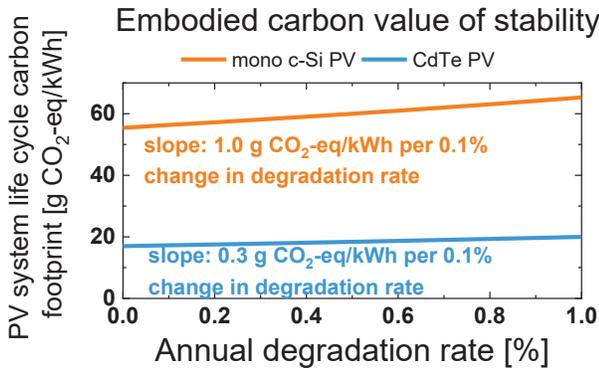
Fig. 2. Life cycle carbon footprint (obtained with ENVI-PV) as a function of annual degradation rate for a ground-mount PV system in a high solar resource location (Daggett, CA, USA) with system lifetime of 30 years. mono-c-Si-PV) Mono-c-Si and CdTe PV are shown with slope indicating the embodied carbon value of stability.
