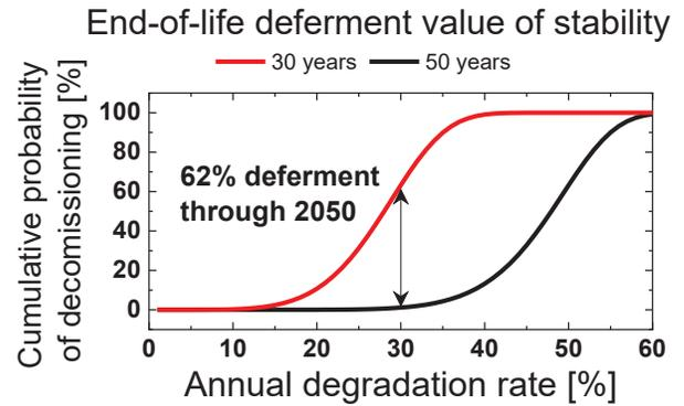
Fig. 3. Probability of PV module loss based on 30 and 50 year average lifetime obtained with Weibull distribution (Eq. 1). Difference between loss curves indicates end-of-life deferment value of stability.
