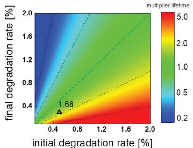
Fig. 4. System lifetime multiplier based on change in annual degradation rate.
