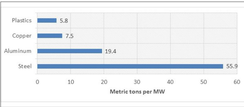
Figure 4. Material fractions of PV power plants [10]
