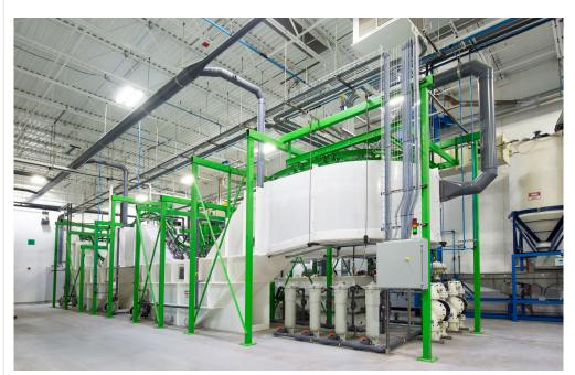
Figure 7. First Solar's third-generation PV recycling technology based on a continuous-flow process
