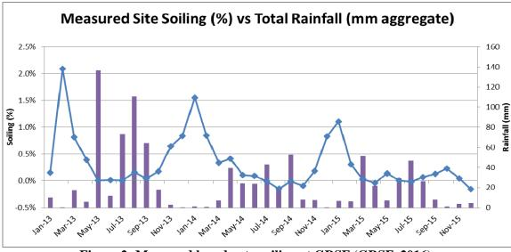
Figure 2: Measured loss due to soiling at GRSF (GRSF, 2016)
