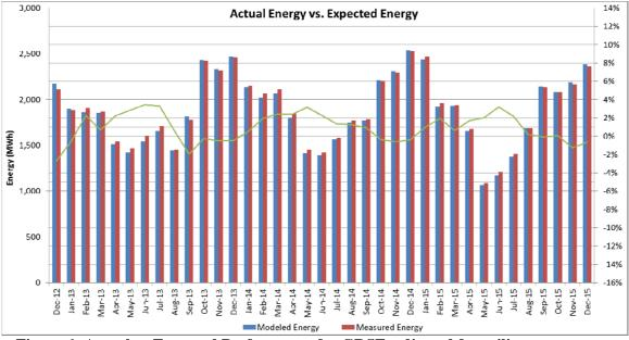
Figure 6: Actual vs Expected Performance for GRSF, adjusted for soiling, spectrum, weather, and outage lost energy (GRSF, 2016)
