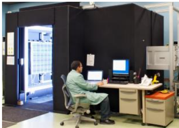
Figure 3.4.3: Class AAA h.a.l.m. flash solar simulator with a standard silicon module.
