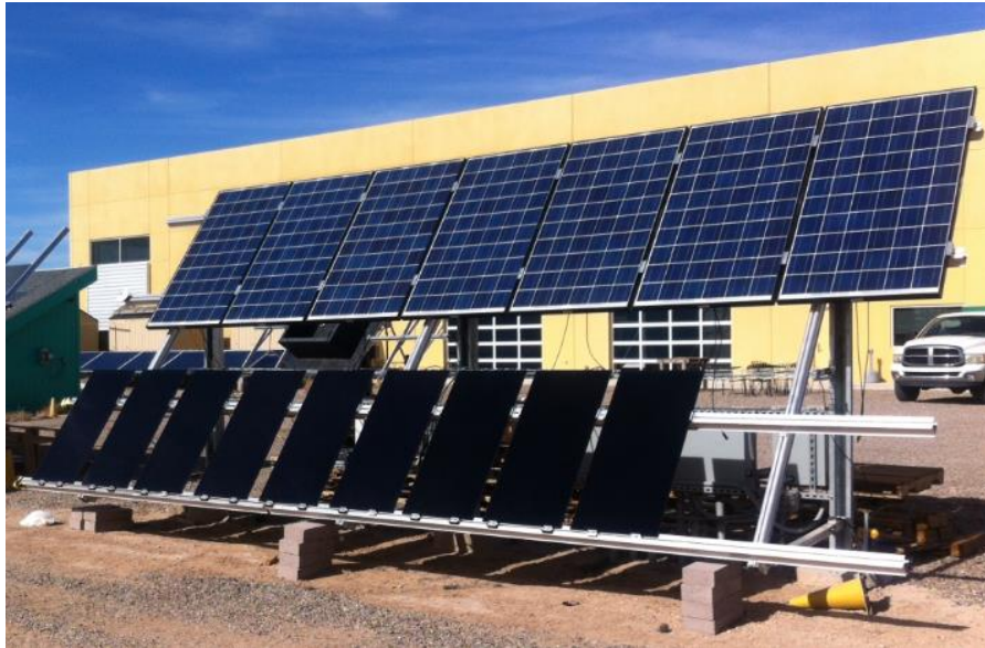
Figure 3.4.1: Fixed-tilt, open air array of FS-395-Plus, FS-4100, and FS-4102-2 modules measured for NMOT.
