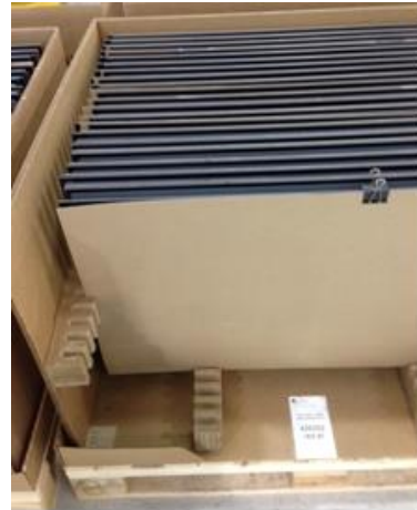
Figure 4: Reusable paper separator to be placed between front faces of modules
