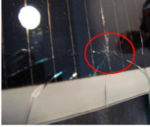
Fig. 2. PV module with fractured glass (impact, edge breakage).
