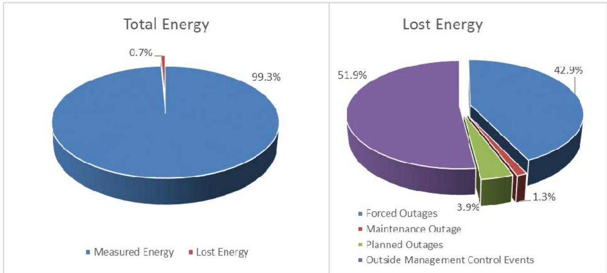
**Figure 5: Lost energy due to outages at GRSF (GRSF, 2016)**
