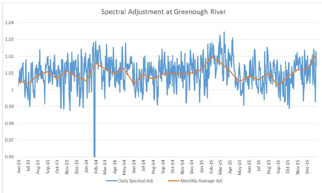
**Figure 4: Estimated spectral shift at GRSF (GRSF, 2016)**
