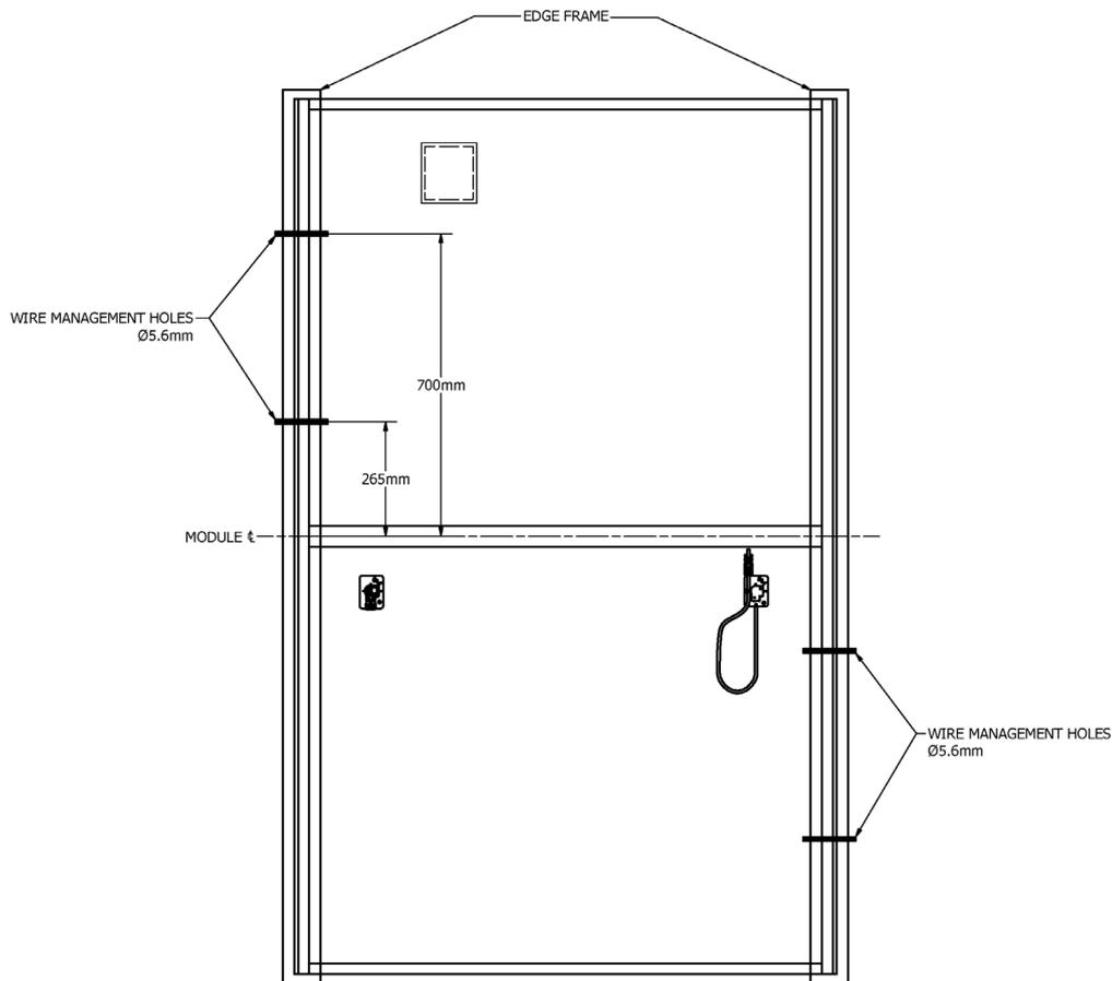
**Figure 10:** The above-ground DC cabling (typically a bundle of harnesses and PV array cables) may be supported by the wire management holes located on the Series 6 module edge frames.
