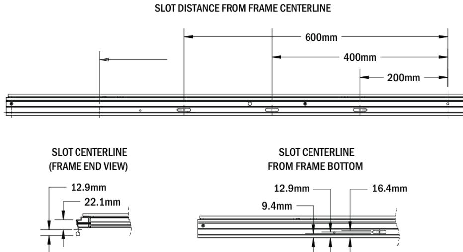
Figure 6. SpeedSlot Detail on Long Edge Frame
