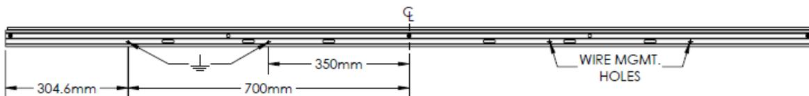
**Figure 9:** Grounding Hole & Wire Management Hole Detail from Frame Center<sup>5</sup>
