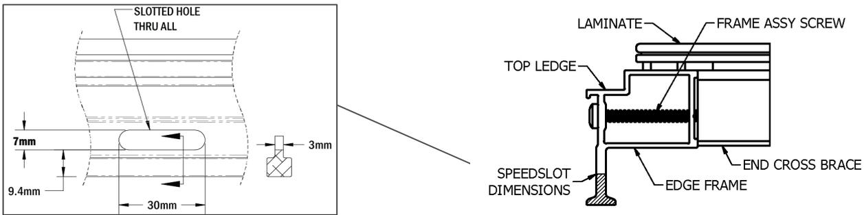
Figure 5. SpeedSlot Dimensions
