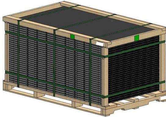
Figure 1: Module Pack Configuration
