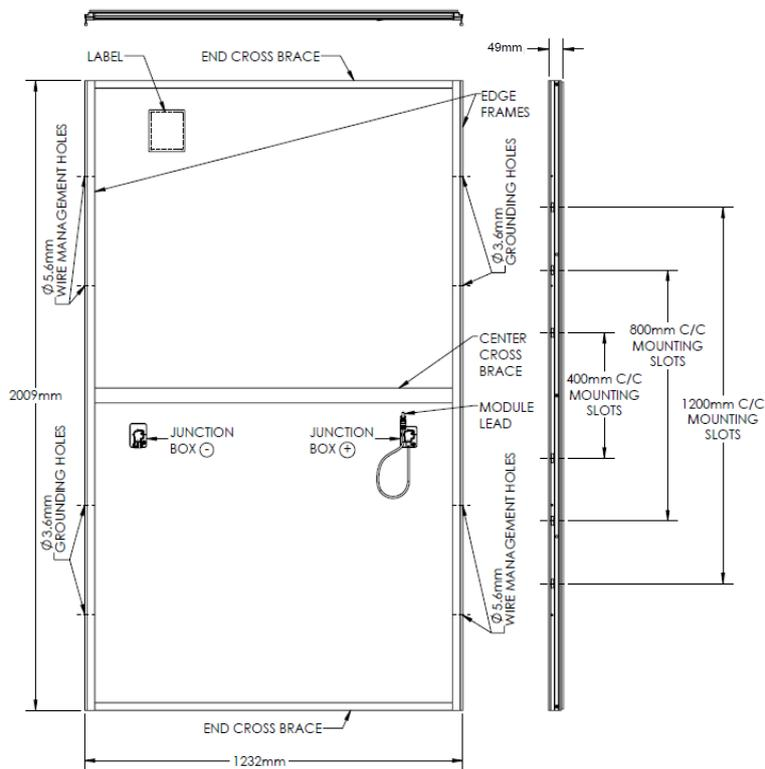
Figure 3: Series 6 Module Mechanical Drawing
