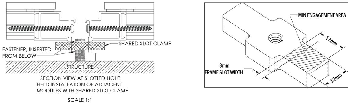
Figure 7: Shared SpeedSlot Clamp Detail
